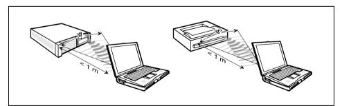
Set up the IrDA transmitter and receiver as illustrated above. The devices may be no more than one meter apart.
