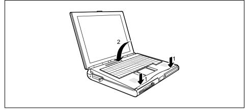
Place the keyboard in the lugs on the notebook (1) and press the keyboard into the bracket provided until it is felt to engage (2).
