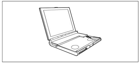
Push your chipcard into the chipcard reader with the chip (contact surface) facing downward.
