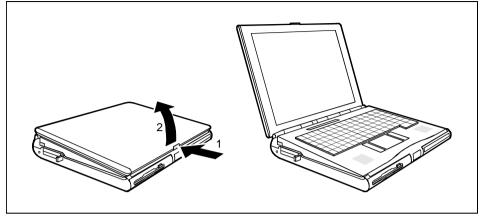
Press the release button (1) and unfold the display upwards (2).
