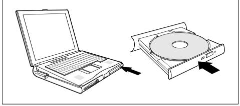
Press the insert/eject button for roughly one second.
